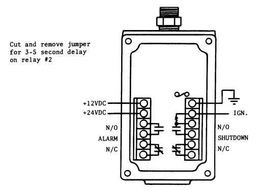
Relay contacts are shown in the normal run condition. Contact state is opposite on fault signal or on loss of 12-24 VDC power. Fault signal causes relay #1 to change state immediately. Relay #2 switches simultaneously (jumper left in place) or with a 3-5 second delay (jumper cut and removed).
