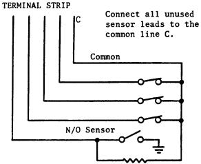
Add 18,000 ohm, 1/2 watt resistor as shown for each normally open sensor that is used with an otherwise normally closed system.
