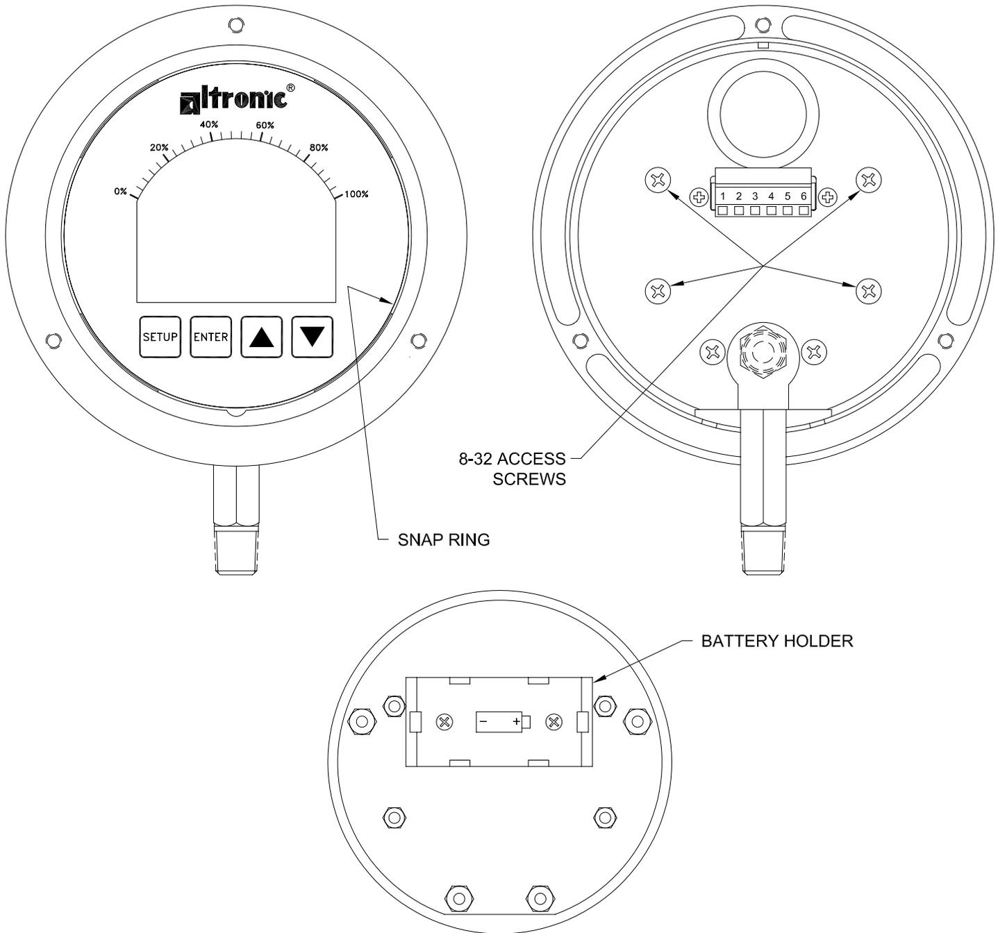
Use 1 each "C" size 3.6 volt high energy lithium battery, Tadiran models TL-5920 or TL-2200 or Saft model LS26500 or equivalent.
