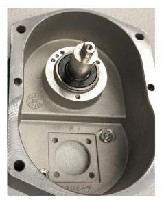
Hole plug screw assembly installed in the location of old Zener.
