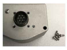
From outside of unit install connector mounting screws and heatsink mounting screw.
