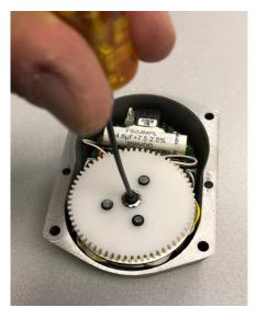
Remove three screws holding the top plate of the pickup coil assembly. Then pull the top plate assembly off.
