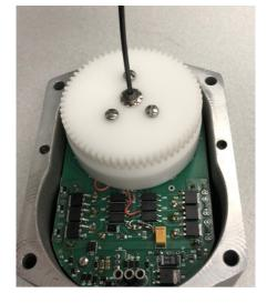
Alternator update is done next. The existing magnet Rotor assembly will be replaced with a new, more powerful, rare earth magnet assembly.
