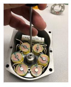
Location of pickup assembly mounting screws.
