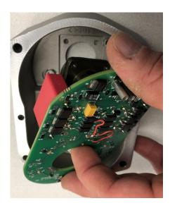
Fasten circuit board assembly to casting using hardware provided, only three screws will align with the tapped holes in machined back cover.
