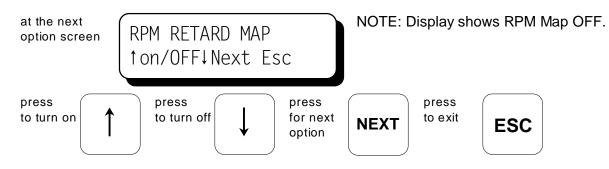
6.4 The Next mode selection can enable or disable the additional retard value controlled by the serial port. To use this option reference form CPU-2000 PI.
