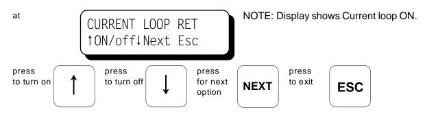
6.3 The Next mode selection can enable or disable the pre-configured retard curve controlled internally by engine RPM. To configure the RPM retard curve, reference form CPU-2000 PI.
