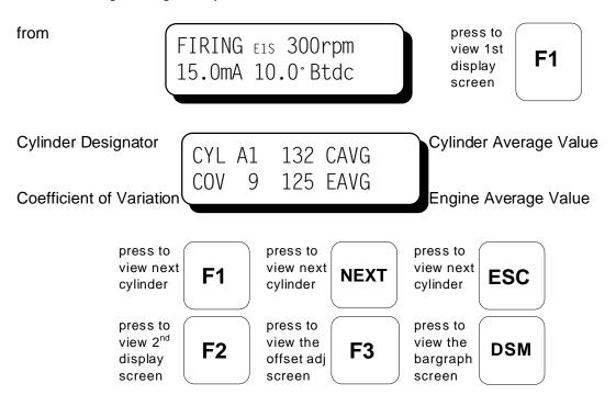
NOTE: Systems with firmware version 2.1 and a 32-output unit with memory engine cycle code "6" or "8" (2 individual outputs per cylinder) will have connector group averages displayed as shown below.
