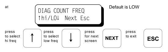
9.13 WITH OPTIONAL DIAGNOSTIC MODULE ONLY: The next screen is used to select the RPM at which to permit the update of the MIN/MAX historical cylinder data array. This feature is provided to avoid the update of the MIN/MAX values when the engine is running below normal loaded conditions.
