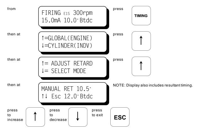
5.3 The increment of timing change is dependent on the number of holes or teeth being sensed. The minimum timing change is equal to "90/N" where N = no. of holes or teeth. EXAMPLE: For 360 holes, the minimum timing change increment is 90/360 = 0.25 degrees.
