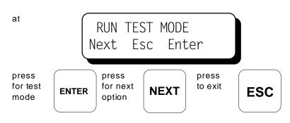
WARNING: The operator MUST fully purge the engine of combustible mixtures prior to selecting the test mode operation. Pressing the enter key again is a confirmation of this action.
