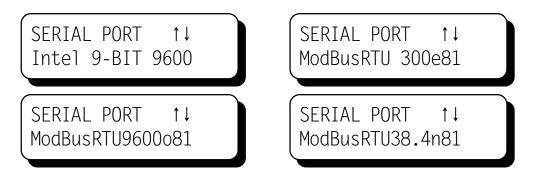
9.9 The Altronic CPU-2000 running firmware version 2.1 includes this screen used to view and select the communication ID-Code or Node-ID. The keypad can be used to select the ID-Code in the range of (0 to 255). Suitable ID-Codes for ModBus are (1 to 247), while suitable ID-Codes for the standard Intel 9-bit communication format are (1 to 254).
