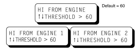
13.7 If the COV reference number is greater than the "HIGH VARIATION" threshold, a diagnostic warning for that cylinder will occur. This test will identify a cylinder whose cycle-to-cycle voltage demand has become erratic.
