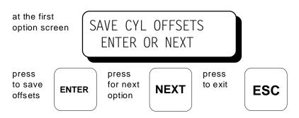
8.3 The NEXT mode function can be used to reset all cylinder timing offset values back to zero (both temporary memory and EEPROM memory).
