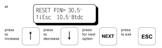
9.6 The next setup screen is used to enable or disable VALUE PROTECTION of all user values in the EEPROM memory. When protection is on, none of the EEPROM settings under the Setup or Timing menus can be changed. This feature can be used to provide limited protection from random changes by inexperienced operators.
