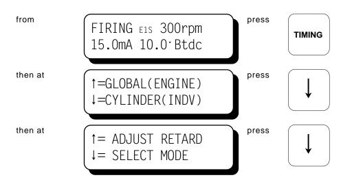
8.2 The first function can be used to save the current (temporary) individual offsets to EEPROM memory. When this is done, the ignition will load these new offset settings every time the engine starts.
