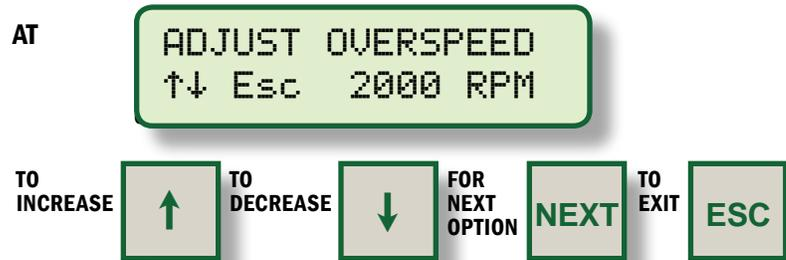
**NOTE:** Adjustment of this parameter should be done while individual cylinder offsets are all at zero.
