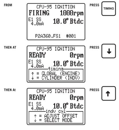
7.3 The individual timing adjustment screen identifies the primary output to be adjusted, and the degrees of offset in use for the output.
