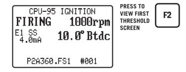
12.2 If the CAVG reference number of a cylinder is below the **LO SPARK VOLTAGE** threshold, a diagnostic warning for that cylinder will occur. This test will identify a low voltage demand condition which may result from a shorted coil, secondary lead or spark plug. To disable diagnostic, set value to zero.
