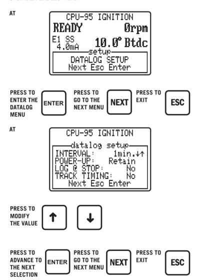
It is possible to setup the system so that any change to the ignition timing will trigger a datalog event (an exception report). Exception reports are automatically generated for alarms or shutdowns.
