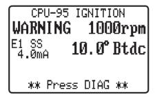
10.3 If the Alarm Out switch is being used to turn on an audible alarm or flasher, the user can acknowledge the alarm as described below.
