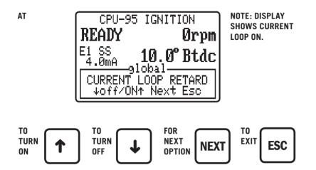
6.3 The next mode selection can enable or disable the pre-configured retard curve controlled internally by engine RPM. To configure the RPM retard curve, reference form CPU-95 PI.
