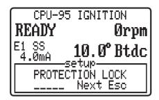
To enter the password press, use the function keys F1, F2, F3, F4 where F1=1, F2=2, F3=3, F4=4 where the number entered is equal to the user assigned five digit password. After the last digit of the proper password is entered, the **VALUE PROTECTION** menu shown above will appear. If the password is not known, press the ESC key to exit or the NEXT key to go on to the next setup menu.
