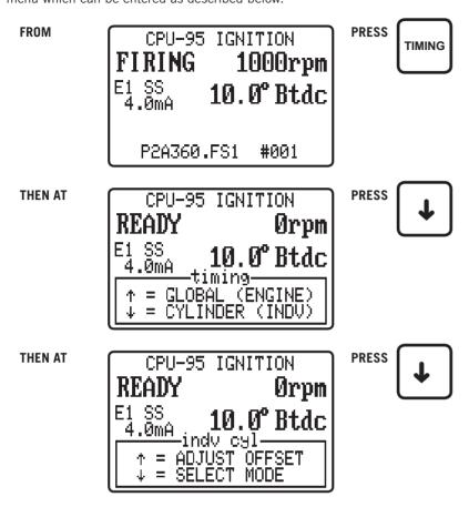
8.2 The first function is used to save the current (temporary) individual offsets to EEPROM memory. When this is done, the ignition will load these offset settings every time the engine starts or reset is pressed. Reference **SECTION 7.0** to adjust individual (temporary) offsets.
