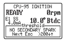
12.5 If the difference between EAVG and CAVG reference numbers is greater than the **LO FROM ENGINE** threshold, a diagnostic warning for that cylinder will occur. This test will identify a cylinder whose voltage demand is too far below the average engine voltage demand.
