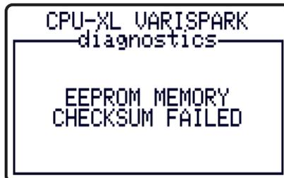
When the programming stored in the Ignition processor is corrupted. This indicates that the Ignition processor must be replaced.
