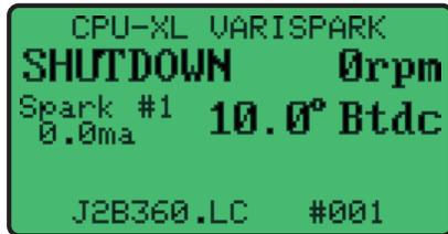
19.9 From the **HOME SCREEN**, pressing the NEXT key allows you to cycle through the configuration comments which describe the configuration of the ignition system.
