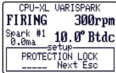
24.6 To enter the password, use the function keys (F1, F2, F3, F4 where F1=1, F2=2, F3=3, F4=4). The number entered is equal to the user-assigned five digit password. After the last digit of the proper password is entered, the **VALUE PROTECTION** menu shown above will appear. If the password is not known, press the ESC key to exit or the NEXT key to go on to the next setup menu.
