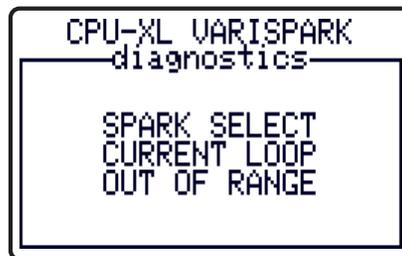
This screen indicates that the voltage detected at the junction module is not within the acceptable range for the requested spark number. This could indicate loose wiring between the Logic/Display Module and Junction/Diagnostic Module or a faulty connector.
