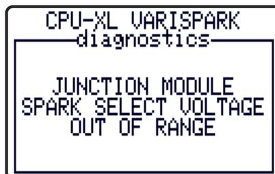
This indicates that the mapping between the spark diagnostics and the actual engine firing order is incorrect and needs to be updated.
