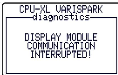
This could indicate a wiring fault or a failure inside the Logic/Display Module.
