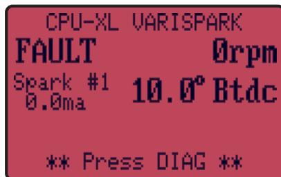
25.2 A diagnostic warning represents the least severe classification of problems. The ignition will continue to fire in the presence of a diagnostic warning. When a warning is detected, several things will occur:
