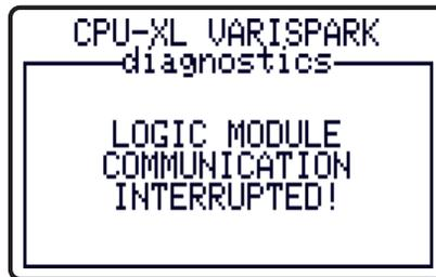
This screen indicates that the Logic/Display Module has lost communication with the Junction/Diagnostic Module. This could indicate a wiring fault between the Logic/Display Module and the Junction/Diagnostic Module or a faulty diagnostic processor inside the Junction/Diagnostic Module.
