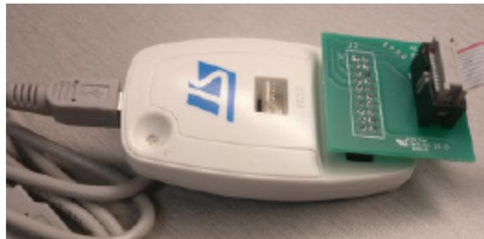
Figure 1.a: ST-Link Programmer Connected to JTAG Board
