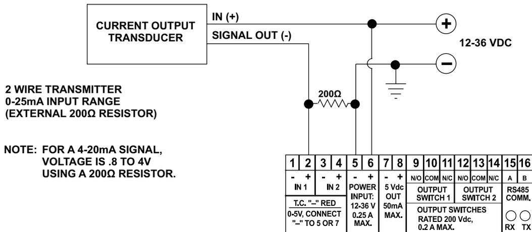
FIG. 15 WIRING DIAGRAM: DC RELAY
