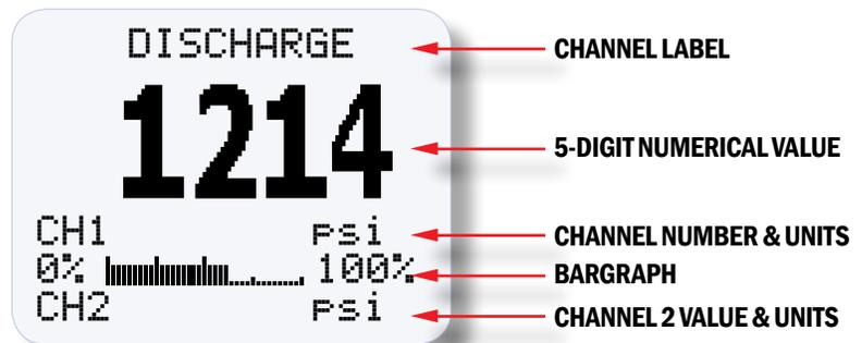
**NOTE:** If one of the inputs is unused it **must be shunted** on the unused input to prevent interference from entering the gauge.
