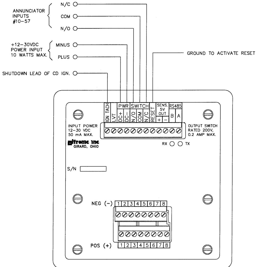
WIRING DIAGRAM – DC RELAY
