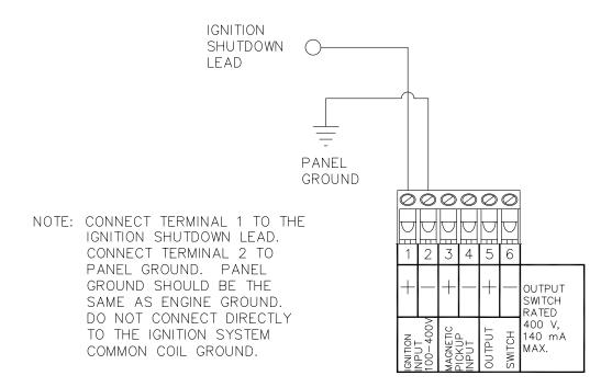
FIG. 5 DTHO-1201/3201 WIRING DIAGRAM POSITIVE GROUND C.D. IGNITION SHUTDOWN LEAD INPUT
