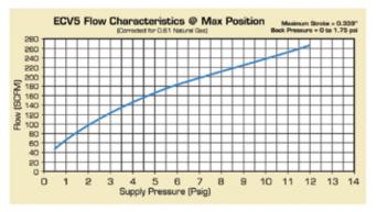
If the injection pressure is zero and the gas flow is 60 scfm, 1 psi of gas pressure is required.
