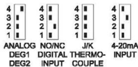
EACH CHANNEL CAN BE CONFIGURED AS N/O, N/C, ANALOG INPUT, THERMOCOUPLE OR 4-20mA.
