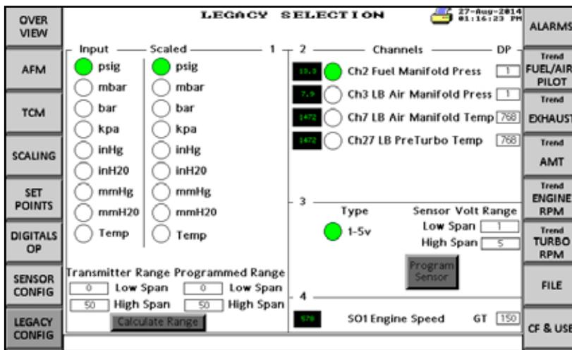
When replacing an existing EPC-200, the end devices require configuration within this screen as described below prior to calibrating any channel.
