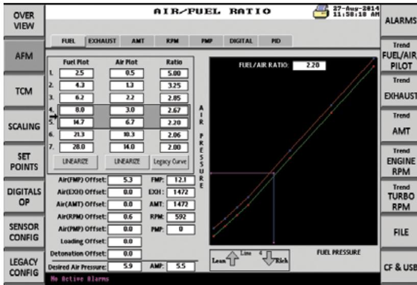
When replacing an EPC-200, enter the existing three point values of the air/fuel curve by pressing the Legacy Curve button.
