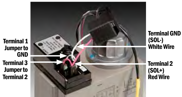
FUEL HARNESS TO ROP CONNECTIONS
