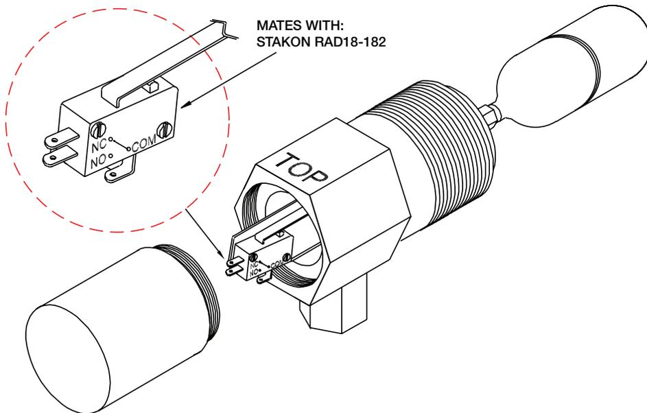
FIG. 3 FLOAT CHAMBER INSTALLATION
