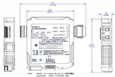
MOUNT TO A 35MM DIN RAIL IN A **SUITABLE** ENCLOSURE. STRIVE TO MOUNT WITH TERMI NALS 7, 8, AND 9 UP TO ALLOW FOR BEST HEAT DIS SIPATION OUT OF THE MODULE WITHOUT TR AVELING THROUGH IT.
