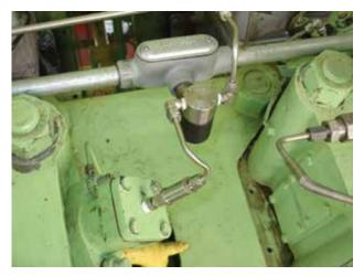
Pneumatic air distributor with pilot-actuated air-in-head valve
