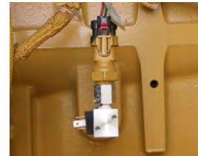
FIGURE VII Manifold Sensor and Harness installed on Sensor By-Pass Kit Assembly
