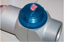
**Single Power Valve** The single power valve will have a seal applied that goes through the top of the
