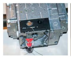
Series A Gas Train The VRF of the series A gas train will have two seals—one applied through the cover of the regulator screw, and one on each side.
